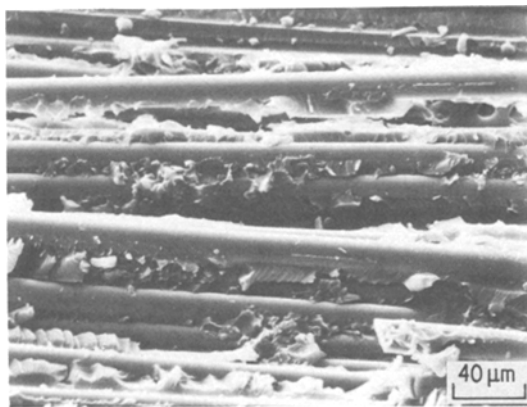
Figure 10 Inter-laminar section showing good interfacial recovery on drying, after exposing at 80° C until a weight increase of 2.5% was reached. × 372
